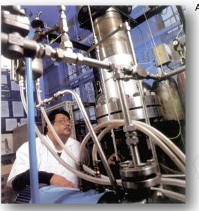
ABSOLV solvent used in the process is proprietary water-based. ABSOLV can capture and separate both CO<sub>2</sub> & H<sub>2</sub>S from Biogas. ABSOLV is regenerated and recycled.
