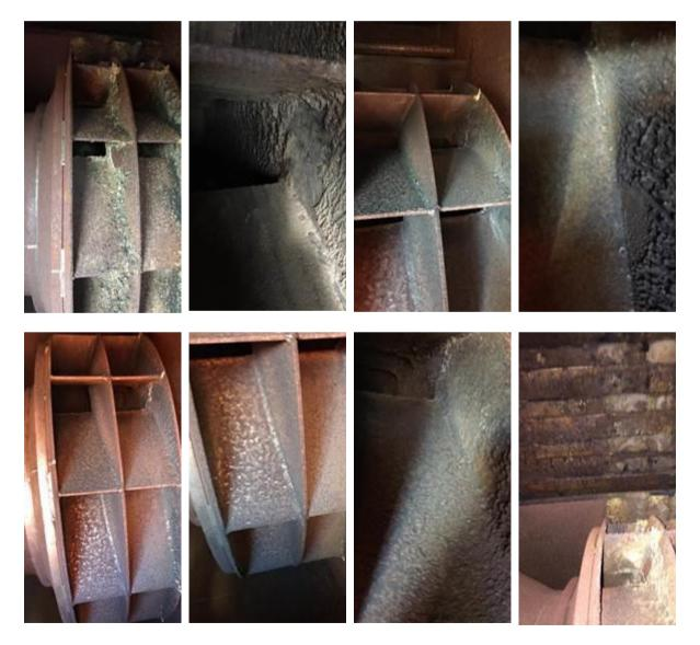
The site team then used an industrial scraper, wire brush and hot pressure washer to then remove the scale from the impellors, photos below for reference show post-cleaning:
